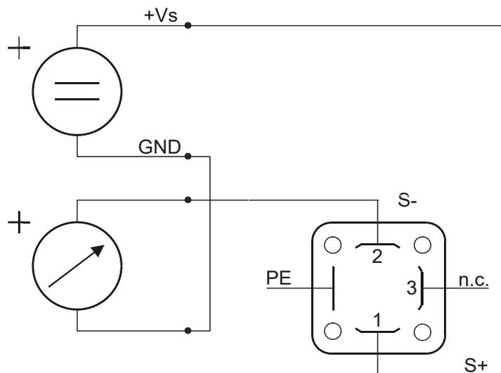
7.4. Cable outlet with M12x1 angle plug electronic options F3x and L3x
