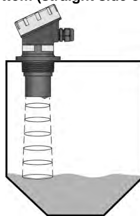
#2 Above an Angled Tank Bottom (straight side only)
